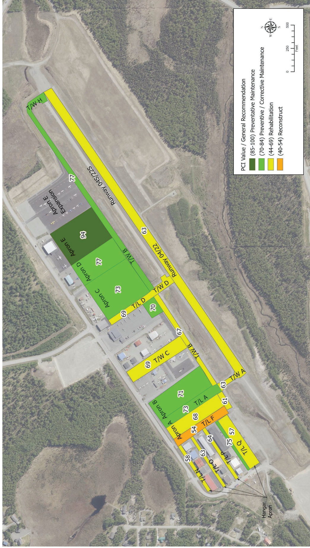
Figure 2-10: Department of Transportation and Public Facilities Pavement Condition Index Results
