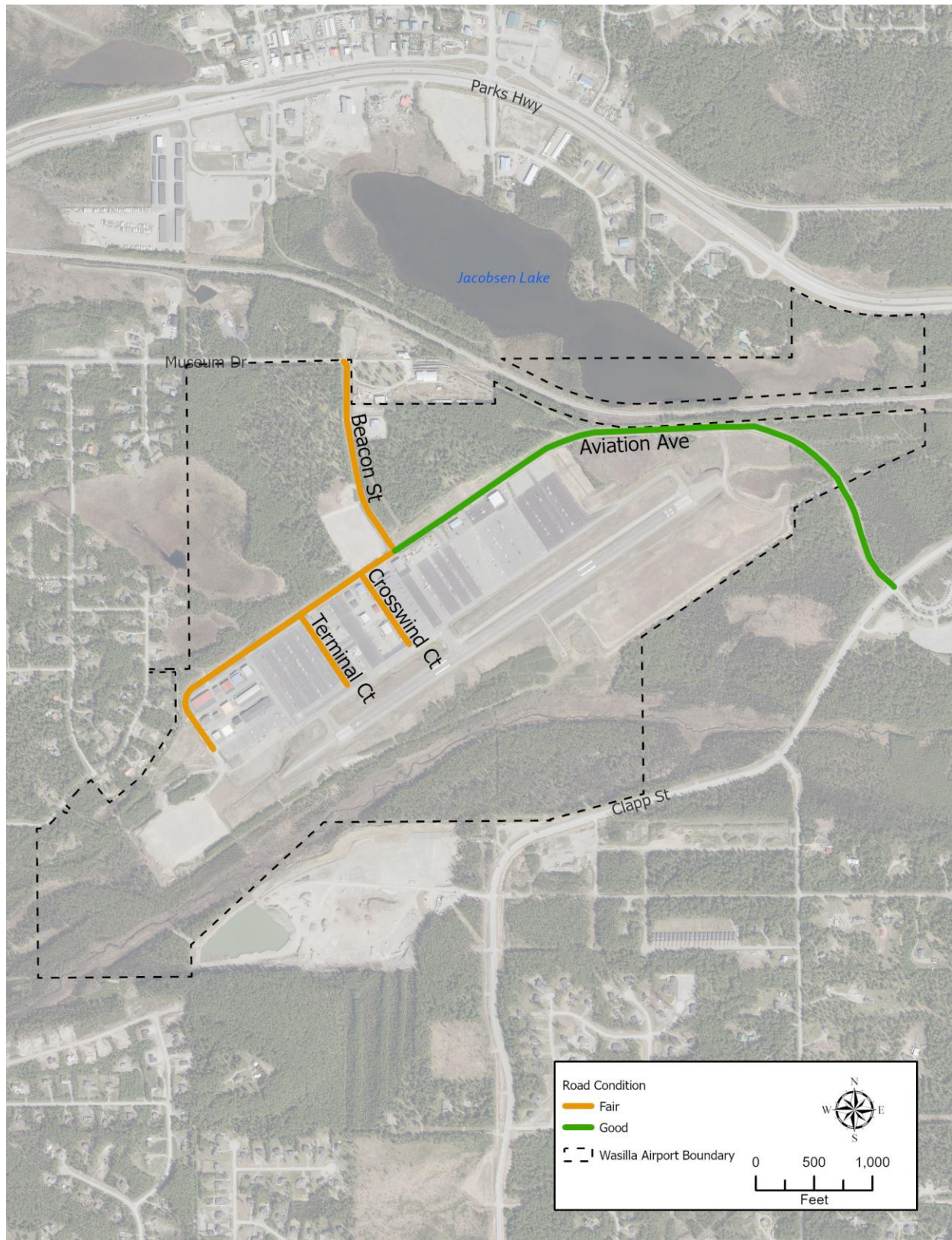
Figure 2-11: Access Road Conditions
